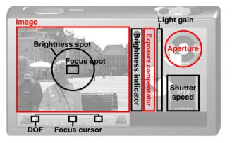
Figure 3.7: Dependence relations among interface elements : All the interface elements are interconnected by causal relationships – visualized by feedforward-feedback interplays.
