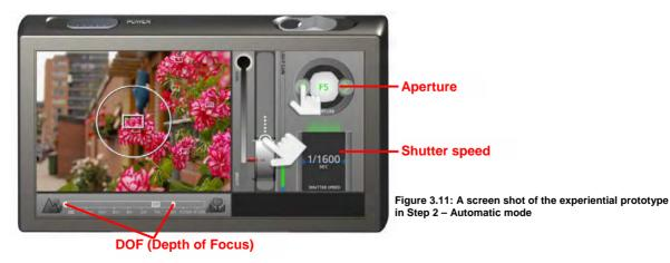
As in Step 1, the Manual mode is activated by pushing Mode control to the right side. In the Manual mode, DOF becomes controllable, and Focus / Brightness spot disappears. Other features are same as in the Automatic mode.
